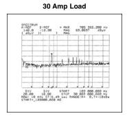
Figure 9-3 — Conducted input noise, with common-mode choke
